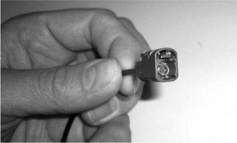
**Fig. 6.37:** Example of a coax cable and coax connector
